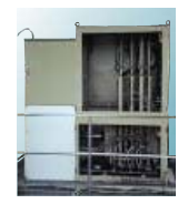
"Parker Scrubber Booth (Water Film Curtain attached B Type)": Paint mist is knocked down to the water surface by means of an abundant water curtain. The curtain surface cleanliness can be maintained because it does not become soiled by the paint.
